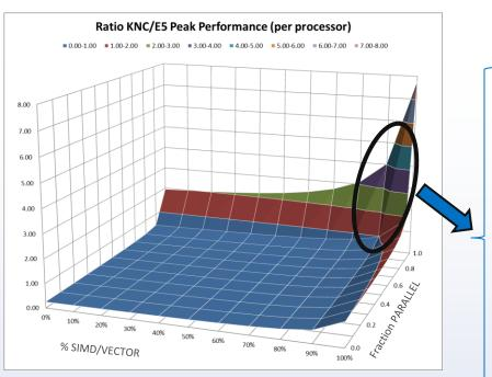
Intel® Xeon Phi<sup>™</sup> coprocessor accelerates highly parallel & vectorizable applications. (graph above)
